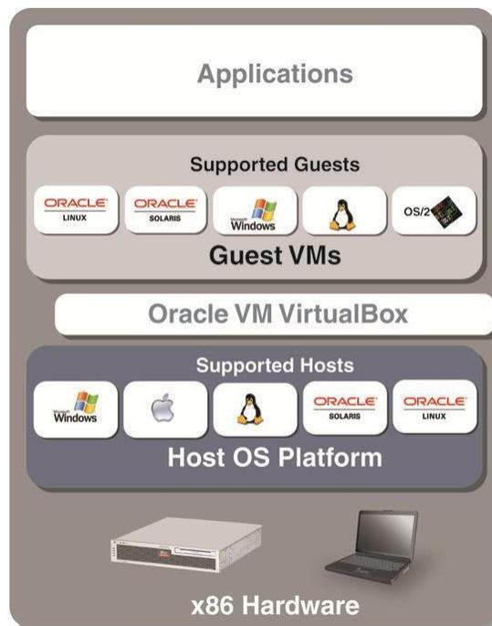
Figure 5.3 architecture of Virtual Box
